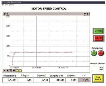
Fig. 6. Motor speed control testing result
