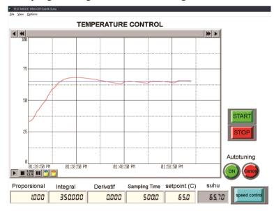
Fig. 7. Temperature control testing result
