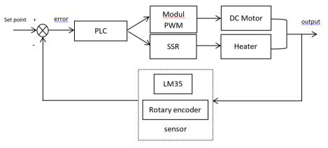
Fig. 1. Block diagram of hardware design
