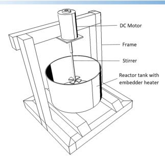
Fig. 2. Biodiesel reactor prototype design
