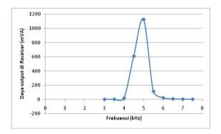
Fig.3.Frequency response of power at the receiver.
