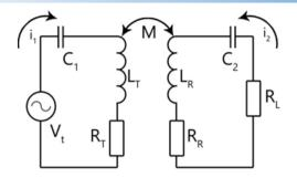
Fig.1.Equivalent circuit of coupled magnetic resonance.
