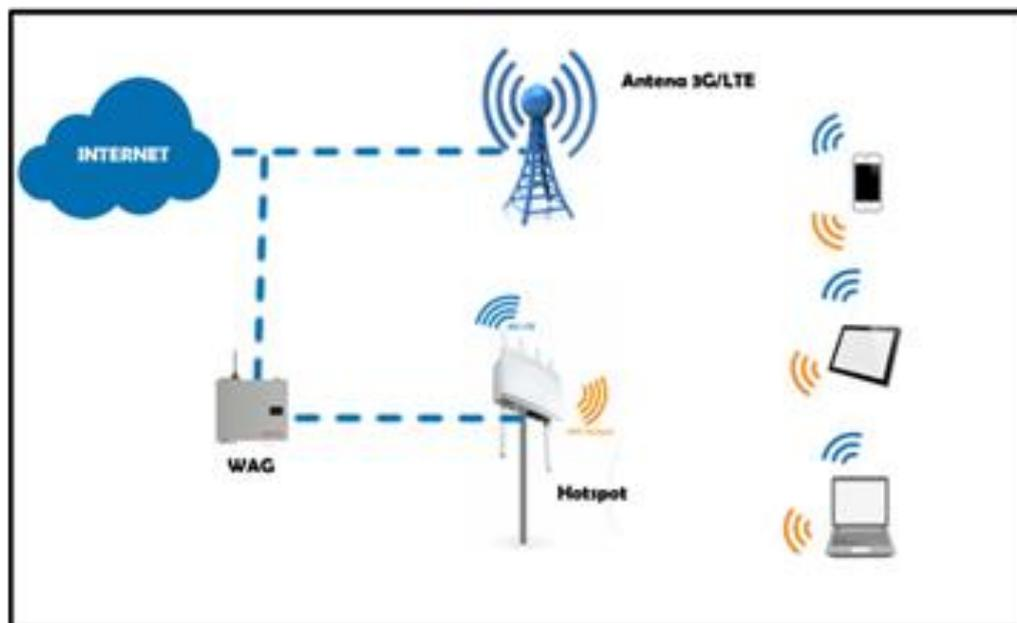
Fig. 1. Wi-Fi offloading network.
