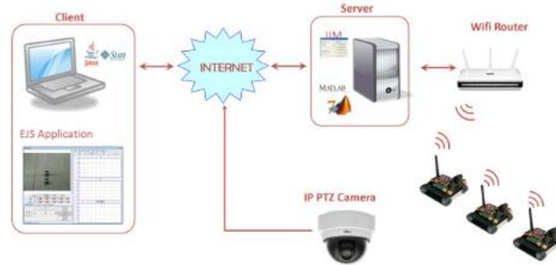
**Fig. 7.**Architecture of the remote lab.
