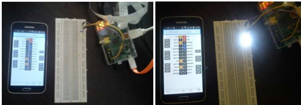
(a) Test Results when the GPIO Pin is Off (b) Test Results when the GPIO Pin is On
