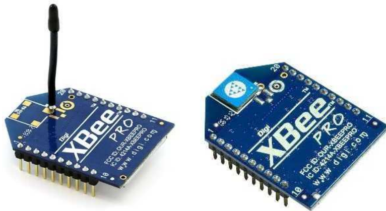
Figure.3 ZigBee Pro S1 Module a (a.Wire Antenna type) and b (b.Chip Antenna type) Antenna type RF Power 63mW / 18 dBm
