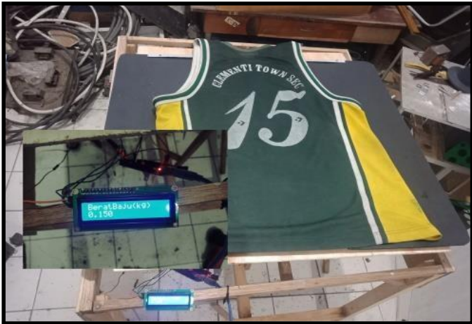
Figure 13. 40S Clothes Load Cell Detection Results
