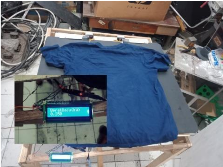
Figure 15. 20S Clothes Load Cell Detection Results
