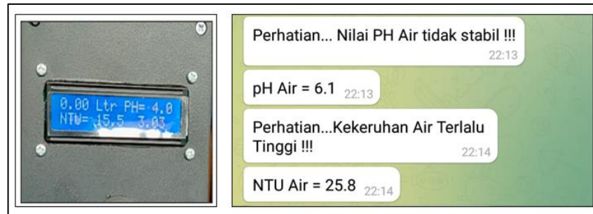
Figure 8. Smart Water Tank Monitoring System
