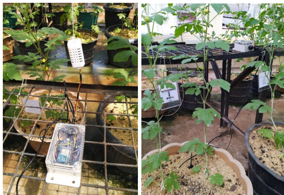
Figure 11. Installation of sensor node v1 in the greenhouse
