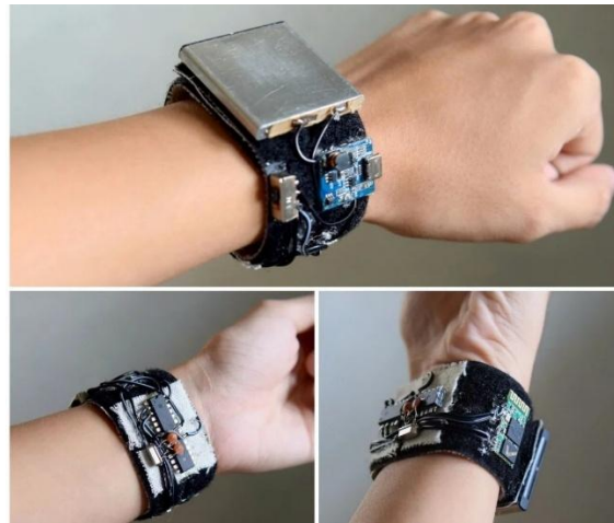
Figure 6. DIY of Wearable Bracelet for Health Monitoring (source: instructables.com/HealthBand )
