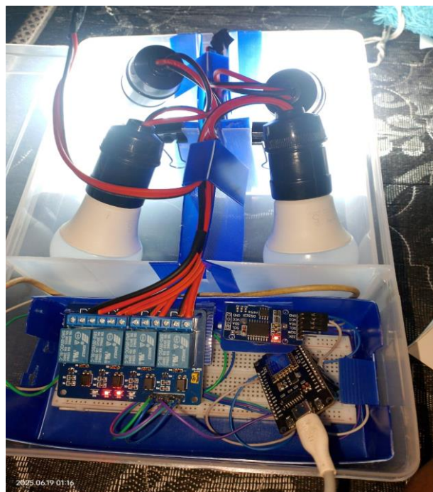
Figure 5. Relay and Node MCU Connectivity, and also Output in the form of Lights
